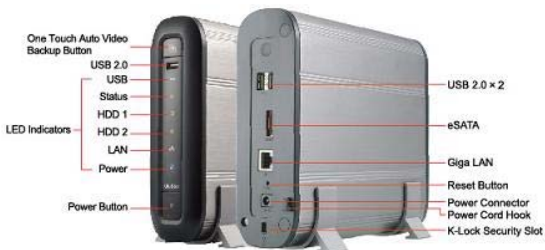
Rys.55 Serwer Q-nap Vio-Stor-101; rejestrator NVR (Network Video Recorder) oparty na systemie Linux.
